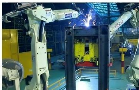
AUTOMATIC WELDING LINE
